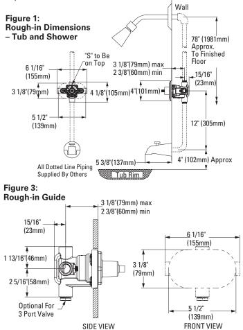
A temperature limit stop limits the movement of the control handle. The standard HydroGuard<sup>®</sup> e420 valve is factory set to deliver tempered water up to 110°F [43°C] with equal supply pressures, with hot water temperature 140°F [60°C], cold water temperature 60°F [15.6°C]
