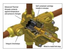
Advanced Thermal Actuation technology maintains a safe and constant output flow despite changes in input temperature or pressure - dramatically minimizing the risks of scalding and facility liability ....
