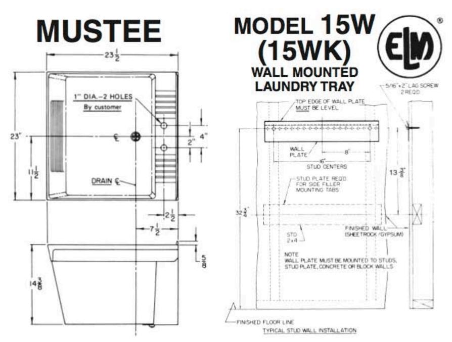
Secure Wall Plate to wall using both 5/16" x 2" Lag Screws. Locate mounting holes 1-1/2" below desired tray height as measured from top edge of rim.
