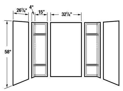
**General:** Furnish and install as shown on plans, DURAWALL® Bathtub Wall model 53, as manufactured by E.L. Mustee & Sons, Inc. The hi-impact thermoplastic wall system shall be 5-piece construction with four formed shelves. One-piece, seamless corner panels with overlapping edges. Uniform color throughout entire thickness of each panel. Color \_\_\_\_\_\_ (White, Bone).
