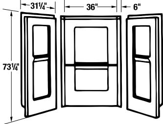
**General:** Furnish and install as shown on plans, 36" square shower, DURAWALL® Shower Walls Model 736, as manufactured by E.L. Mustee & Sons, Inc. Shall be 3-piece, molded fiberglass wall with minimum thickness of 125 mils and mounts direct-to-studwalls. Includes center panel with molded-in shelves and two side panels with molded-in shelf. Self aligning panels use a tongue-and-groove connection. Shall meet ANSI Specification Z 124.1.2. Color\_\_\_\_(White, Bone).
