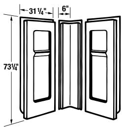
**General:** Furnish and install as shown on plans, 36" neo-angle shower, DURAWALL® Shower Walls Model 736C, as manufactured by E.L. Mustee & Sons, Inc. Shall be 3-piece, molded fiberglass wall with minimum thickness of 125 mils and mounts direct-to-studwalls. Includes center panel with molded-in shelves and two side panels with molded-in shelf. Self aligning panels use a tongue-and-groove connection. Shall meet ANSI Specification Z 124.1.2. Color\_\_\_(White, Bone).
