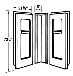
**General:** Furnish and install as shown on plans, 38" neo-angle shower, DURAWALL® Shower Walls Model 738C, as manufactured by E.L. Mustee & Sons, Inc. Shall be 3-piece, molded fiberglass wall with minimum thickness of 125 mils and mounts direct-to-studwalls. Includes center panel with molded-in shelves and two side panels with molded-in shelf. Self aligning panels use a tongue-and-groove connection. Shall meet ANSI Specification Z 124.1.2. Color: White.
