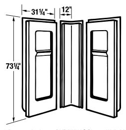
**General:** Furnish and install as shown on plans, 42" neo-angle shower, DURAWALL® Shower Walls Model 742C, as manufactured by E.L. Mustee & Sons, Inc. Shall be 3-piece, molded fiberglass wall with minimum thickness of 125 mils and mounts direct-to-studwalls. Includes center panel with molded-in shelves and two side panels with molded-in shelf. Self aligning panels use a tongue-and-groove connection. Shall meet ANSI Specification Z 124.1.2. Color: \_\_\_\_\_ (White, Bone)
