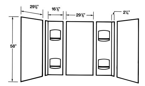
**General:** Furnish and install as shown on plans, DURAWALL® Bathtub Wall model 952, as manufactured by E.L. Mustee & Sons, Inc. The hi-impact thermoplastic wall system shall be 5-piece construction with four formed shelves. One-piece, seamless corner panels with overlapping edges. Uniform color throughout entire thickness of each panel. Color: White. Weight 23 lbs
