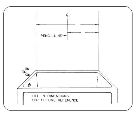
2. Accurately measure tub spout and handle(s) hole location on alcove side wall and transfer dimensions to one of the remaining flat panels. Measure from front edge of bathtub. You may want to make a template (use shipping carton) to check hole layout before you cut holes into side panel. After you have double checked your measurements, using the proper size drill or hole saw, cut out holes for outlets. Cut from front (finished) surface.
