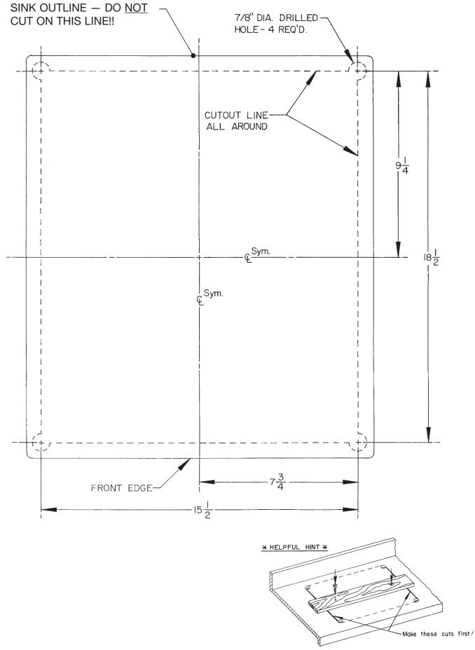
After making cuts along sides of cutout, secure a board as shown to prevent cutout from possibly damaging countertop or prematurely dropping.
