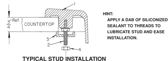
6. Apply a bead of clear siliconized sealant\* (not furnished) all around the underside of the rim in the molded-in groove — See Detail Drawing. Place **Hospitality Sink** into the countertop cutout, secure from the underside with hardware provided. You will need a 7/16" socket or wrench to secure Mounting Nuts (4) in place. Wipe away any excess sealant that squeezes
