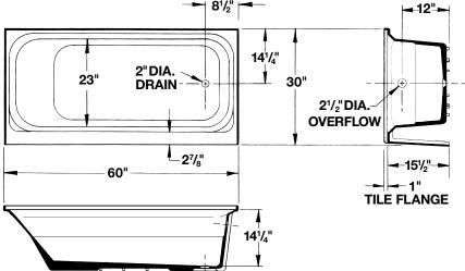
**General:** Furnish and install as shown on plans, TOPAZ® bathtub as manufactured by E.L. Mustee & Sons, Inc. Shall be a fiberglass 30" x 60: right hand or left hand Model \_\_\_\_\_\_. Construction shall be molded, reinforced fiberglass using matched metal molds under extreme heat and pressure. Shall meet ANSI Specification Z-124.1.2. Color: \_\_\_\_\_\_ (White, Bone, Biscuit) Weight: 74 lbs. Install in compliance with local codes.
